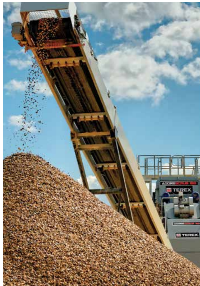
Integral Aggregate Stockpiling Conveyors
