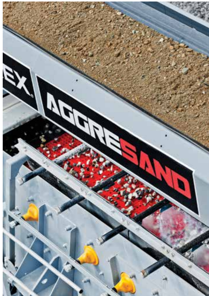
Aggregate Screen Fitted with Isolated Spraybars
