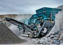
High capacity single toggle jaw Chamber size: 1000mm x 600mm (39" x 23.6")
