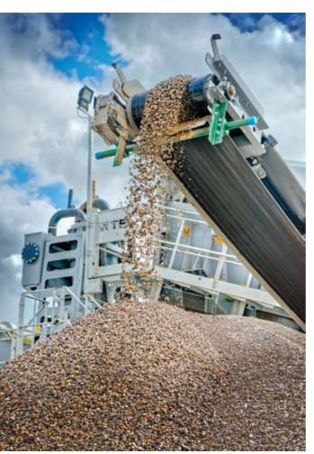
Integral Aggregate Stockpiling Conveyors
