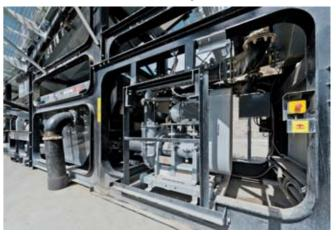
Centrifugal Pumps, Roll out for Service Access
